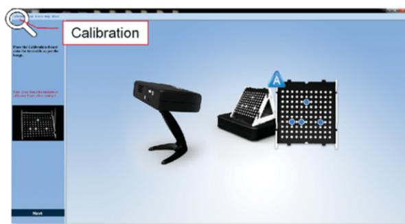
Before your first scan or if you move, reposition, or drop your scanner, you should run the calibration process.
