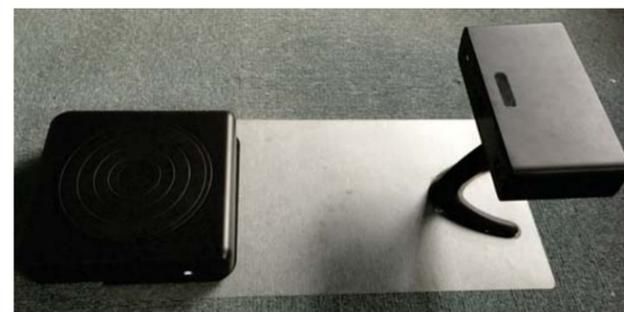
Set the turntable and scanner in the outlines on the positioning sheet.
